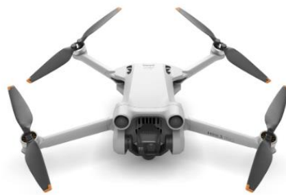
Model: DJI Mini 3 Pro Colour: Light Grey Unfolded size: 251x362x70mm Weight: 249g
