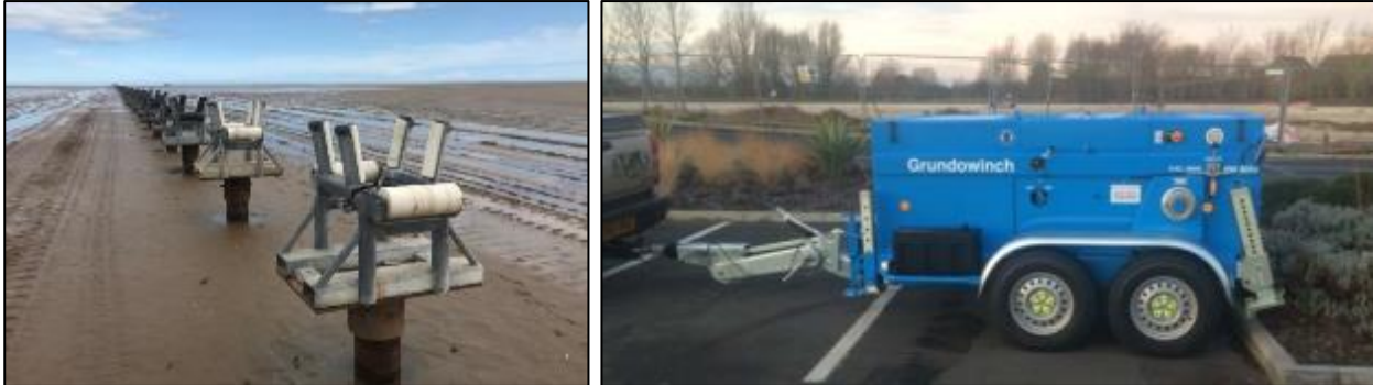
Figure 4.10: Indicative Example piled roller highway (left), typical mobile winch
