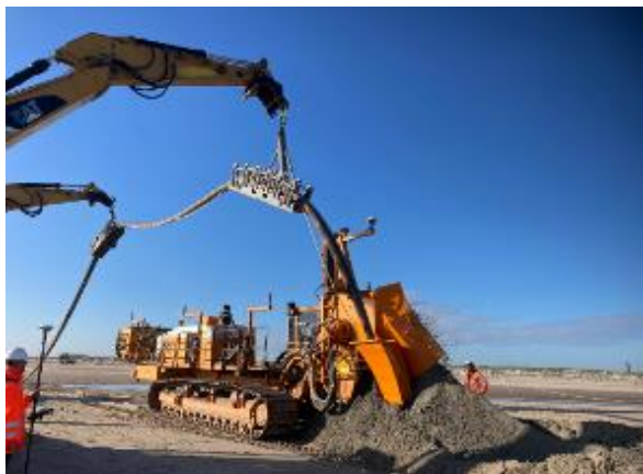
Figure 4.23: Tracked cutter trencher for onshore and intertidal burial
