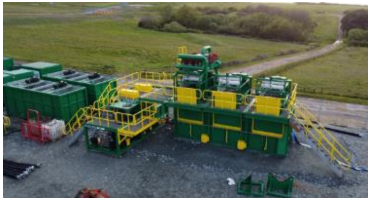
Figure 6.5: Drill Fluid Recycling Plant (typical)
