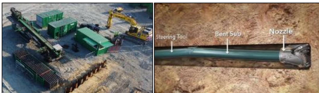
Figure 4.13: Typical drilling rig and pilot drilling assembly
