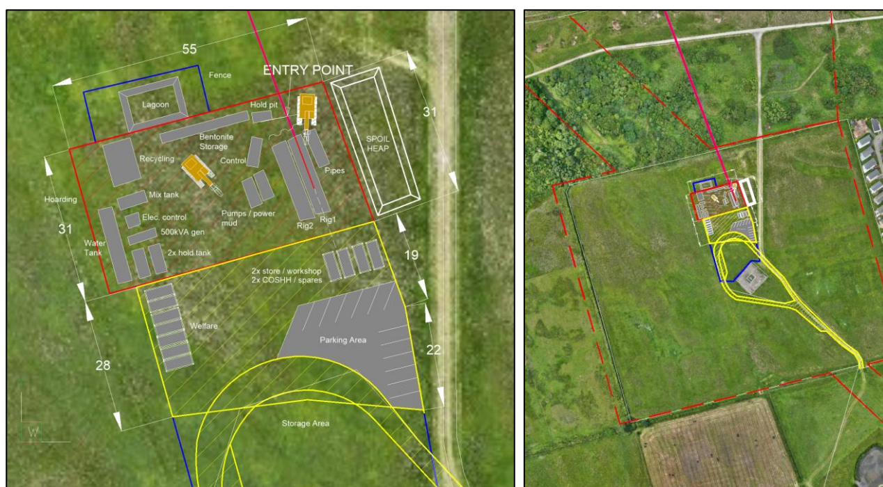
Figure 4.5: Non Indicative Entry Site Set-up for HDD works. Detailed view on the left, overview of Warren Farm on the right.
