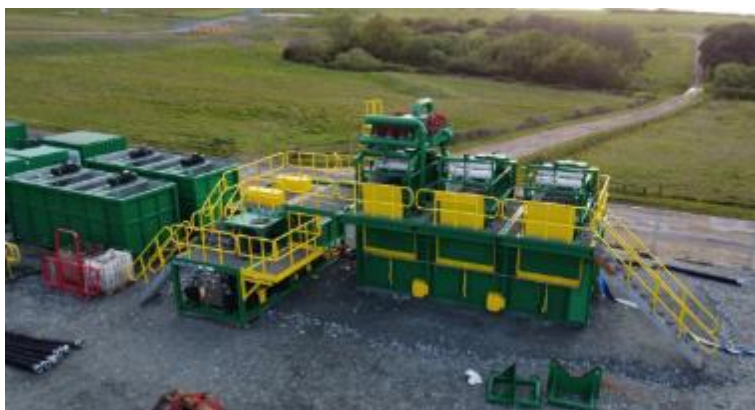
Figure 7.3 Drill Fluid Recycling Plant (Typical)
