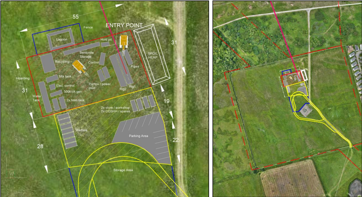
Figure 4.10 Non Indicative Entry Site Set-up for HDD Works. Detailed View on the Left, Overview of Warren Farm on the Right
