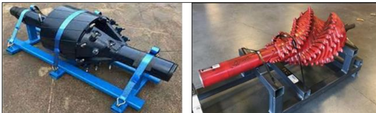
Figure 4.19 Rear Reaming Assembly
