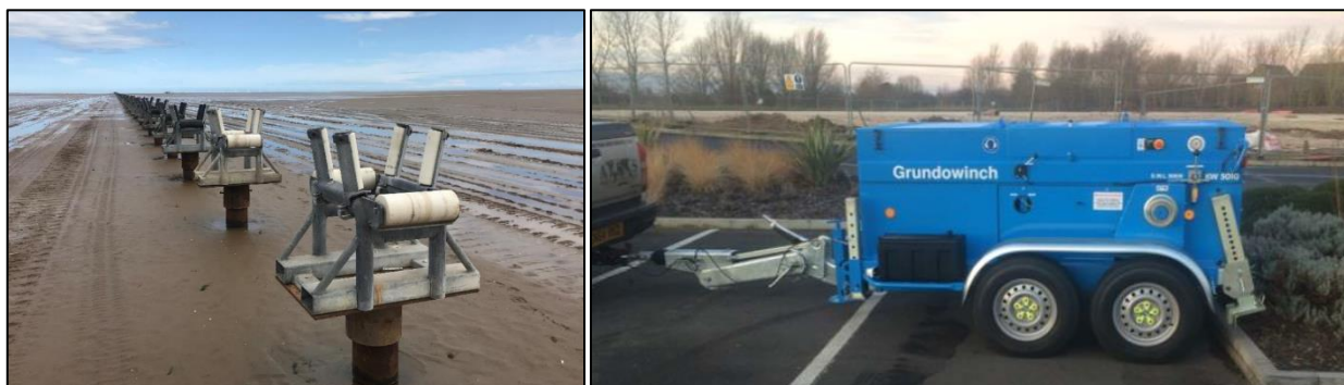
Figure 4.15 Indicative Example Piled Roller Highway (Left), Typical Mobile Winch
