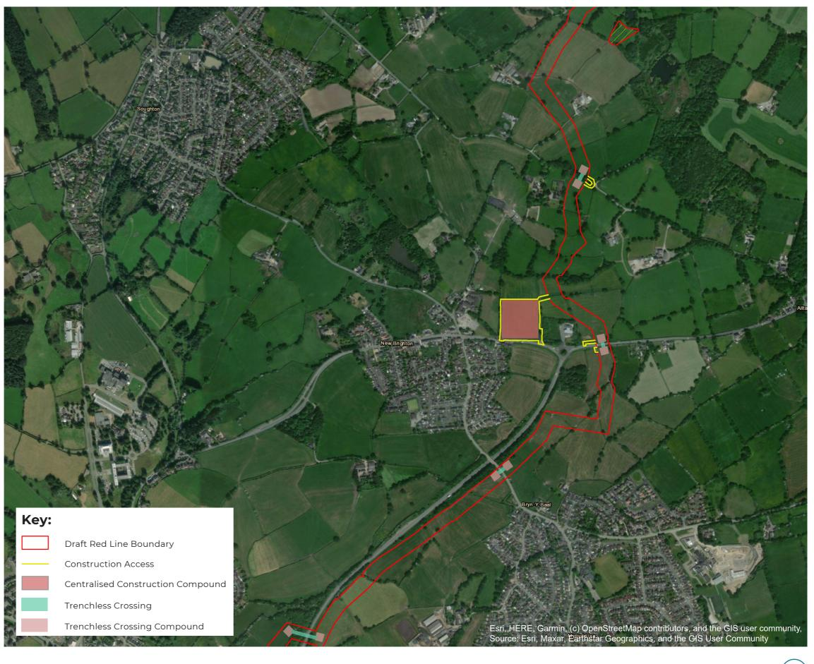
In this section, the Padeswood Carbon Dioxide Spur Pipeline runs northwards towards the A55 and an area of Ancient Woodland. At the road crossings and under this area of Ancient Woodland, the spur pipeline will be installed using trenchless crossing techniques to minimise impacts and avoid the need to close and divert the A55.
